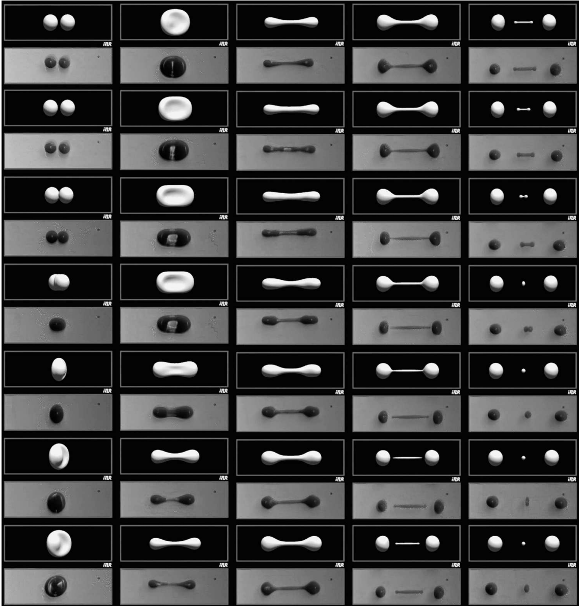
Abbildung 7.12: series of pictures taken from an animated gif (taken from [3]); above the simulated collision, below the real collision
